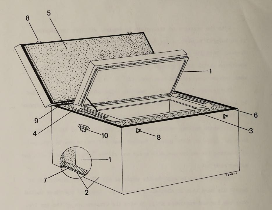
Figure 1. Construction of field ice box.
